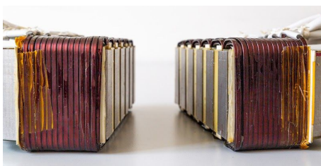
Linear Induction Motor of the 2020 Swissloop Pod
